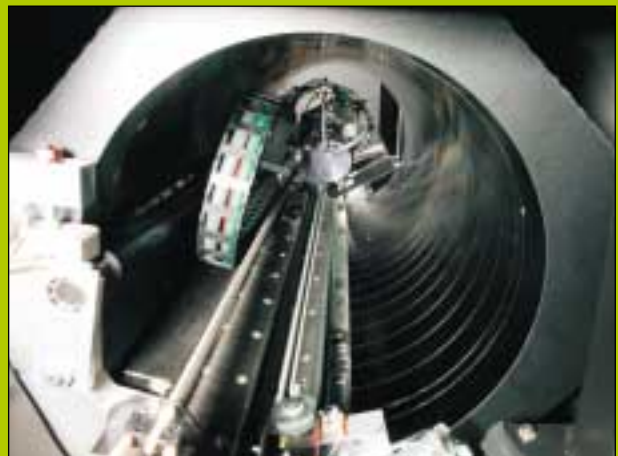
Internal drum with in-line punch for high quality production.
